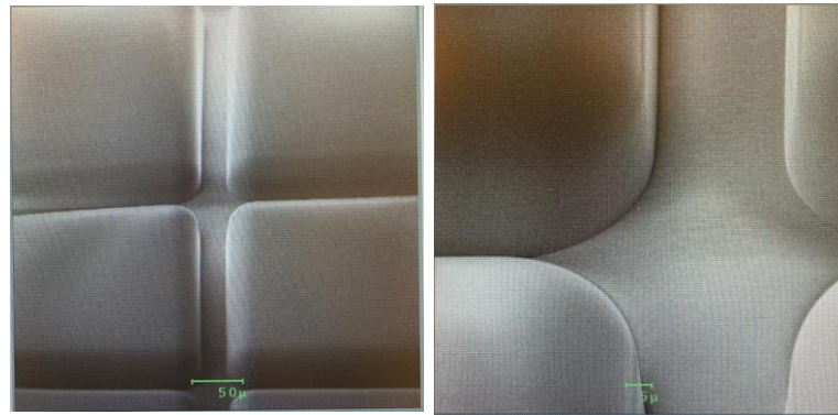
No visible cracks after PECVD
